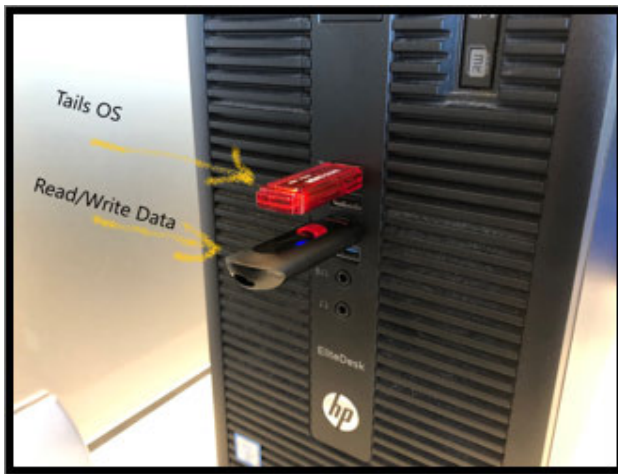
Figure 5: Air Gap boot disk and Read/Write Sneaker Net Data Transfer Flash Drive
